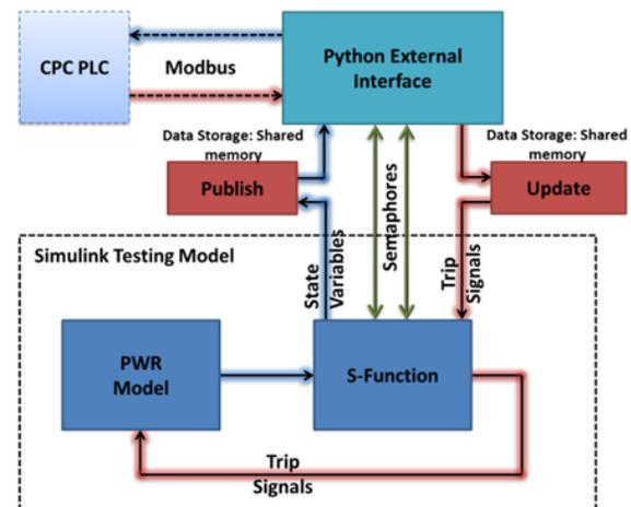
Fig. 2. Developed data transfer interface for linking Simulink to external PLCs.<sup>3</sup>
