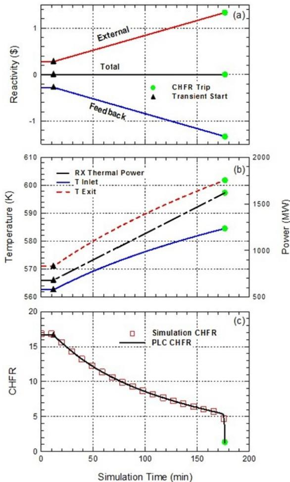
Fig. 3. Comparison of CPC CHF trip simulation data to those of the Simulink based model.
