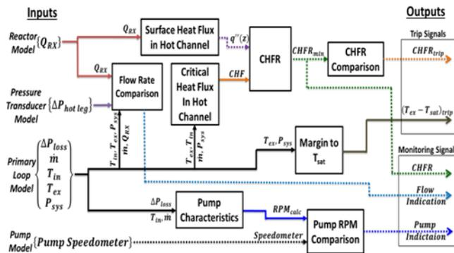
Fig. 1. CPC functional block diagram.
