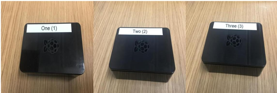
**Figure 2.7:** Raspberry Pi units used in the network response identification tests. Raspberry Pi number 1 is the same unit which was used in the real and emulated PLC comparison.
