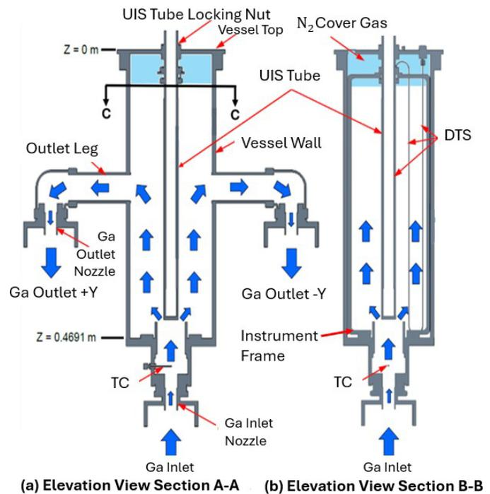
Fig. 2 Cutaway view of the upper plenum of the GaTE experimental facility.
