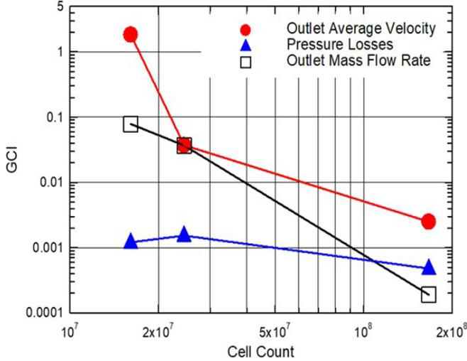
Fig. 4 Comparison of the effect of the numerical mesh refinement on the GCI.
