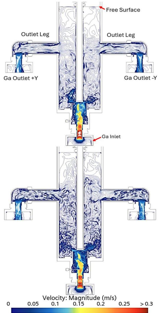
Fig. 5 Comparison of the Calculated Flow Field and Velocity Contours using Coarse (Top) and the Fine (Bottom) Mesh Grids.
