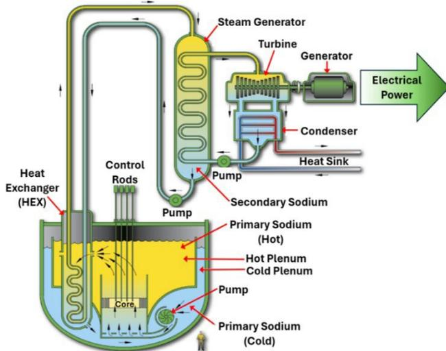
Fig. 1 A Layout of a Pool Type SFR [1].
