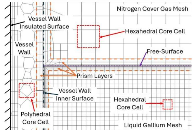
Fig. 3 Numerical Mesh grid in liquid Gallium and near solid surfaces.
